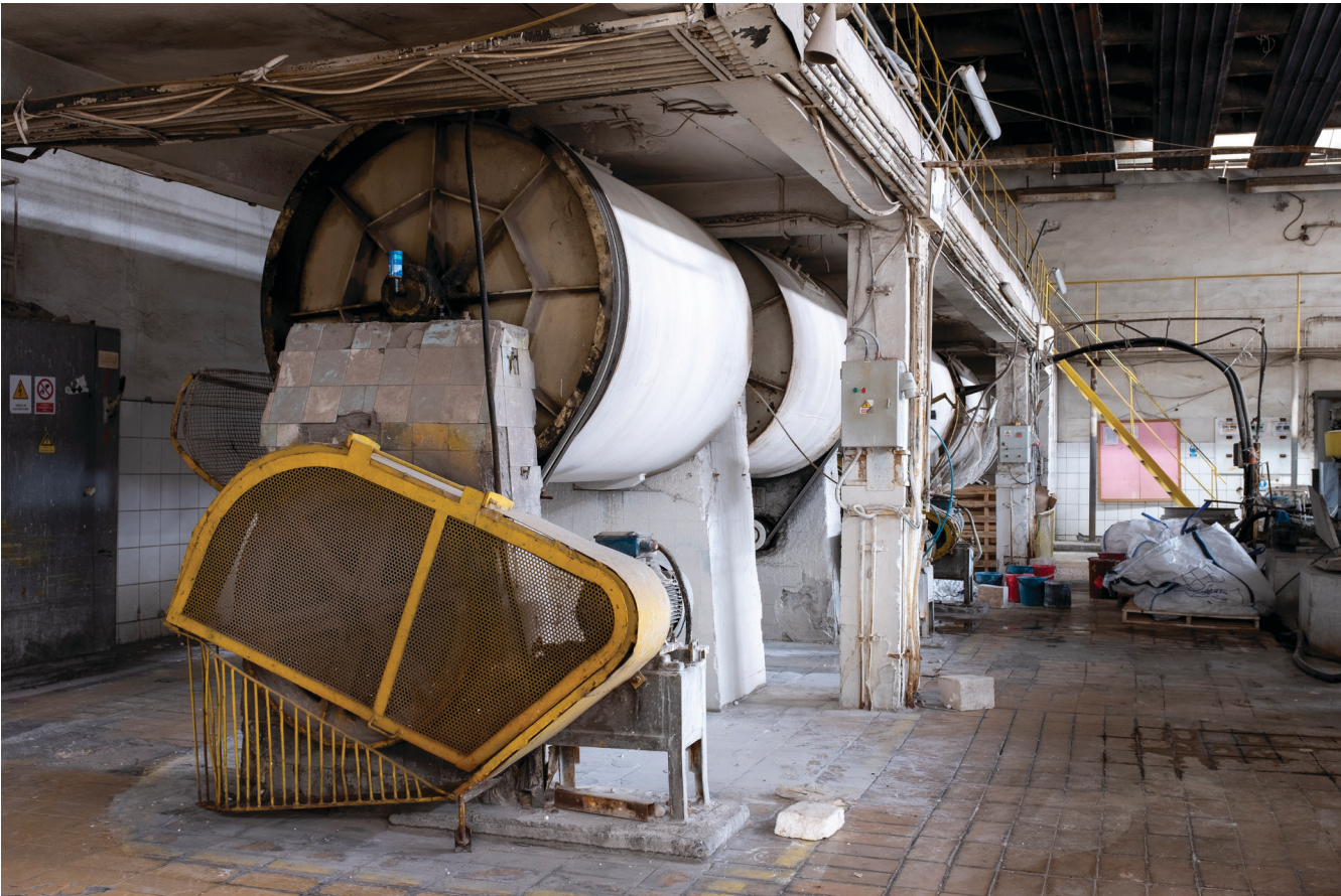
Milling cylinder that uses hundreds of alumina balls for grinding the raw materials.
