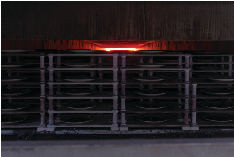
One of the four ovens that IPEC uses to fire ceramic plates, which is 80 meters long and runs continuously.
