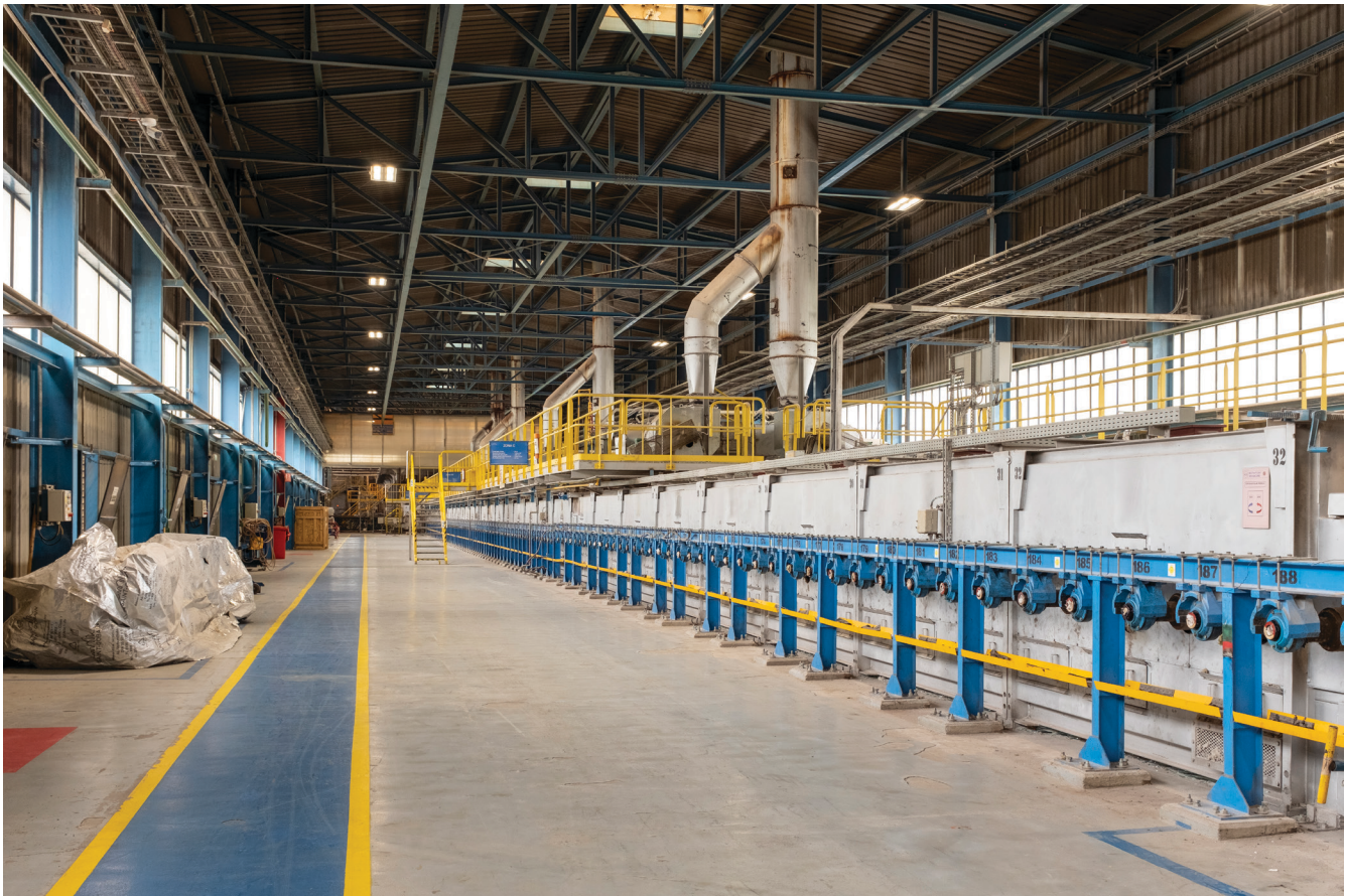
The glass panels are produced on a continuous production line, from furnace casting to cutting and stacking.
