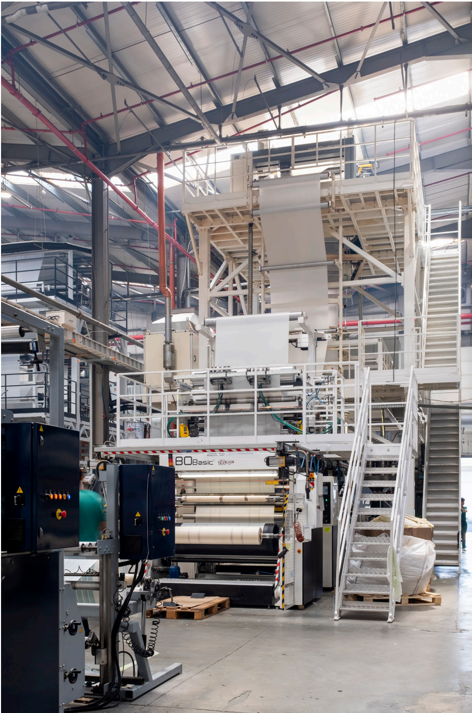
The production line for thin bioplastic film is designed as a vertical system.
