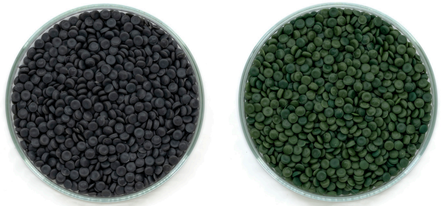
Bioplastic granules obtained by recycling the waste sheets resulting from bag production. The colour of the granules comes from the pigment used to print text on the bags.
