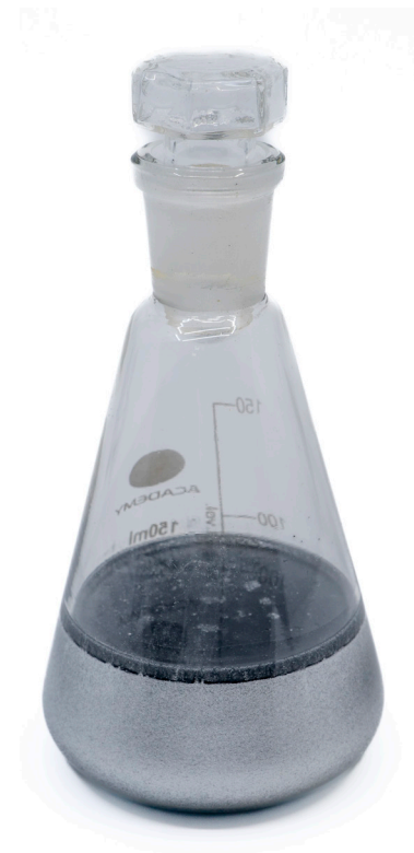
NAME ALBADECOR liquid aluminum PRODUCT APPLICATIONS Decorative pigments COMPOSITION Aluminum 40%, water 60% INDUSTRY Paints, plastics CLIENTS Paint manufacturers ANNUAL PRODUCTION QUANTITY 3600 tons PRODUCTION TIME / ITEM 24h WORKERS/ON PRODUCTION LINE 50 PRODUCTION PROCESS Semi-automated
