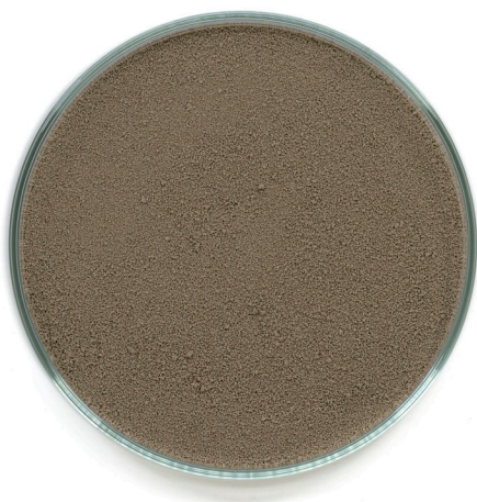
Clay mixture for production of ceramic plates.
