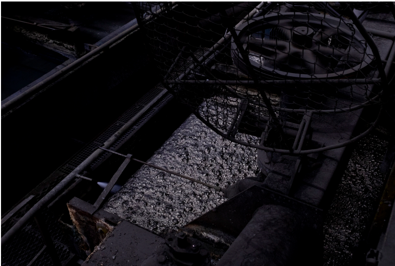
The foam that is formed contains copper and represents the moment when the ore separates from the tailings.
