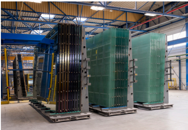
The final glass sheets, each measuring 12 by 6 meters, are ready to be shipped to production facilities.
