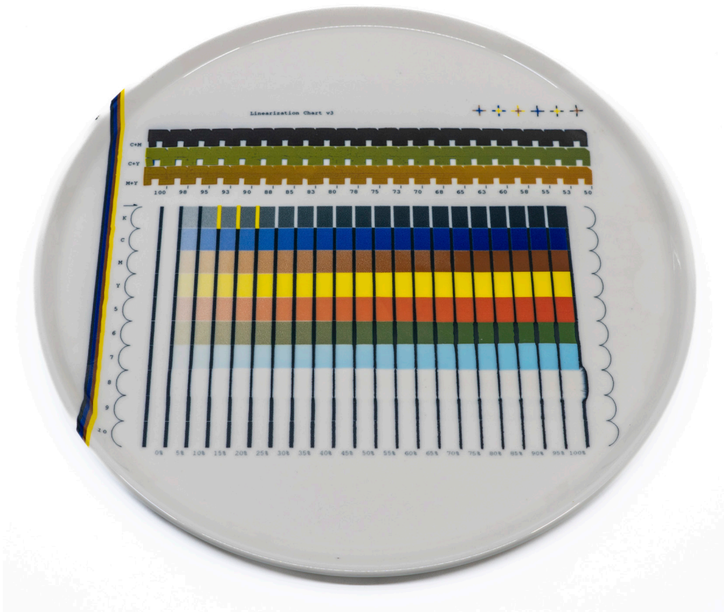
High-resolution digital colour test on a glazed plate used in IPEC production.
